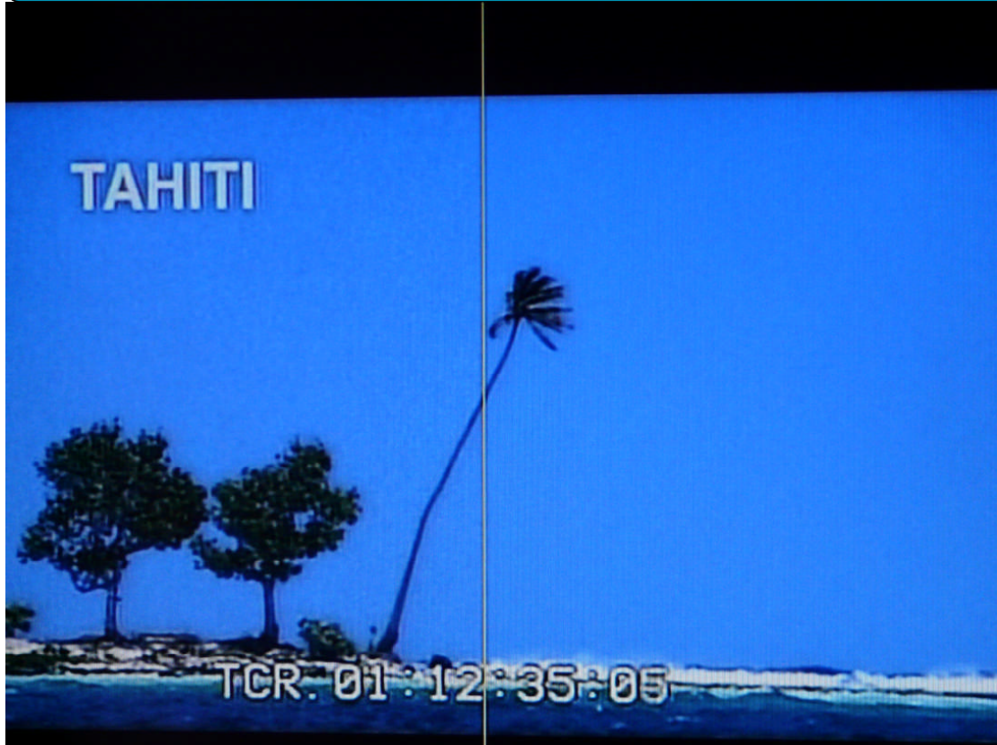
Figure 1 PT12 noise reduction (left side image is NR off; right side image is medium noise reduction)
