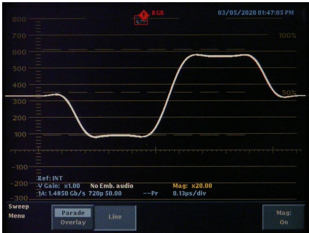
Figure 13 Demodulated horizontal sync waveform.
