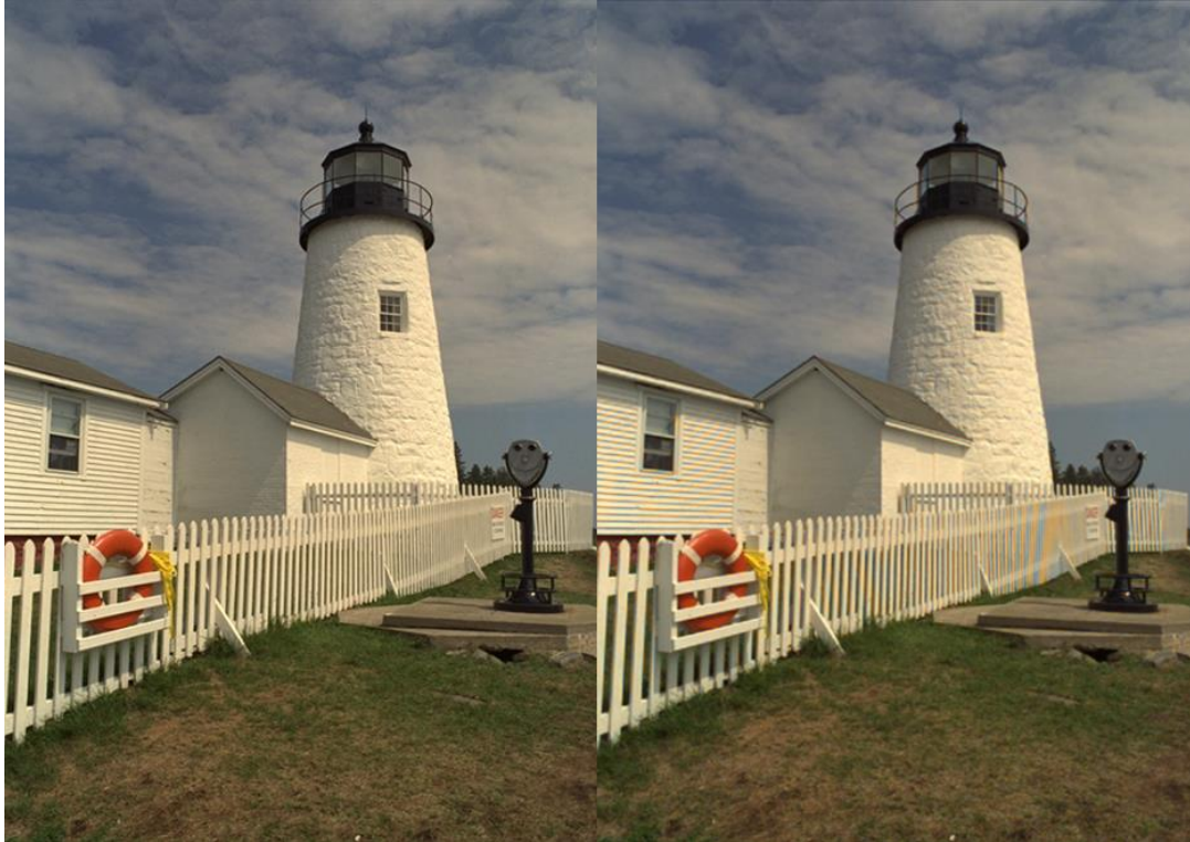
Figure 3 Left: Original full resolution image. Right: Image after Bayer demosaicing.
