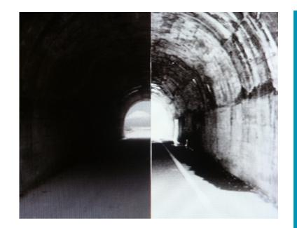
The original image on the left (above) is a view through a tunnel. The bright tunnel opening means that any other details are 'crushed' into the blacks. On the right is the histogram equalised image from the SM03 – now all the details on the walls of the tunnel can be seen.
